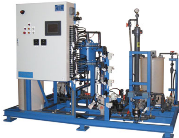
Figure 11: Amine Purification System for CO 2 Sequestration
