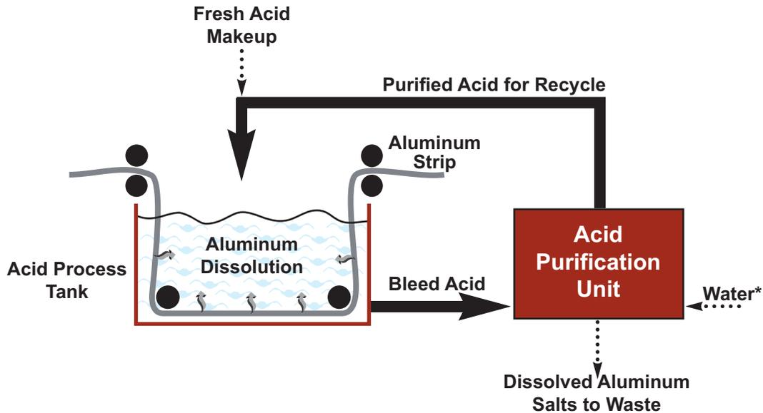
\* some applications require only water, other applications require water and alternate acid for regeneration (typically sulfuric or hydrochloric acid).
