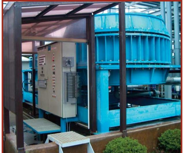
Decationization and Purification Unit (DPU) installed on Capacitor Foil Process in Japan
