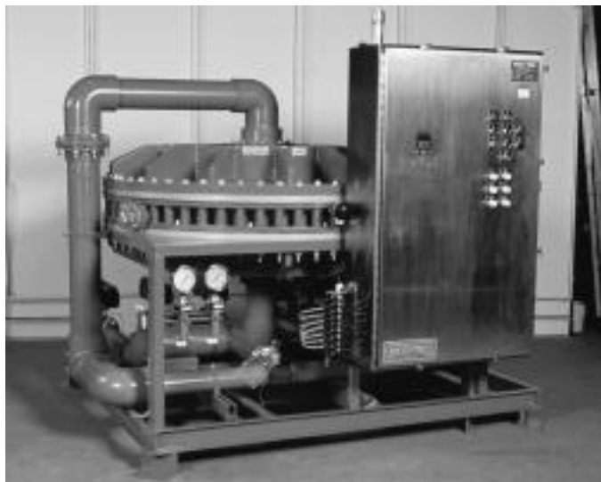
Figure 8: Recoflo Ion Exchange Unit Installed at Champion, Canton NC
